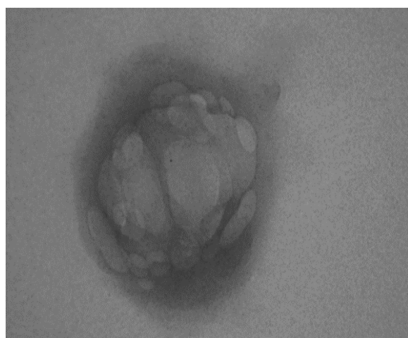
Figure 7: Transmission Electron Microscope image of nimodipine-loaded transferosomes.
